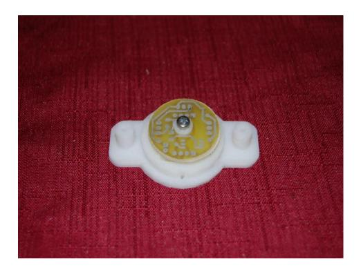
Place the sensor dome over the base and screw into place with  $3 \times \#2 \times 6.4$ mm self tap screws. Ensure that the screws are at right angles to the dome base as the dome may crack if the screws are not in line with the holes.
