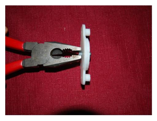
Feed PCB cable through cable exit duct on dome base. Use M3 bolt and plastic washers to fasten PCB to dome base.
