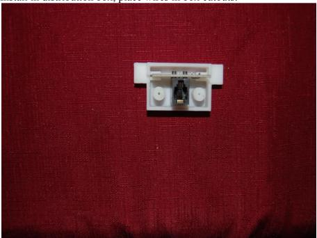
Fit box top and fasten with 2 x #4 x 19mm self tap screws:
